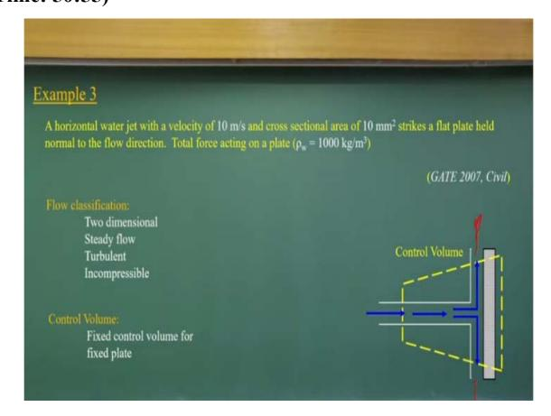
[A horizontal water jet with a velocity of 10 m/s and cross sectional area of 10 mm<sup>2</sup> strikes a flat plate held normal to the flow direction. Total force acting on a plate ( $\rho_w = 1000 \text{ kg/m}^3$ )] Flow classification:
