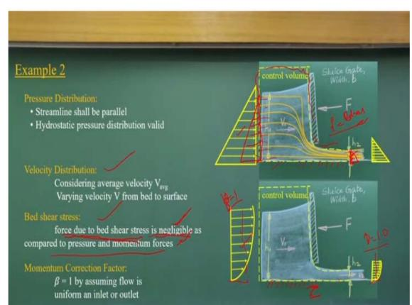
Now, first is pressure distribution. Now, if this is my control volume, first I need to draw the streamlines. So, as it expected that the streamlines will be like this, so as actual fluid valve if you have it could be like this, if the follow of actual fluid valve, if I follow it, it could be like this. So, we should consider the control volume such a way that, at a slow par distance such a way that all the streamlines should be the parallel, okay.
